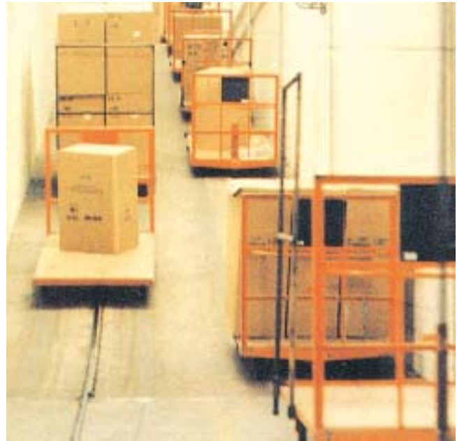
Towline conveyor system for carton transport
