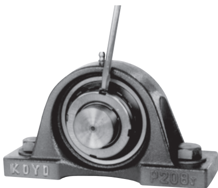
Fig. 14.8 Bending outer tab of washer (Locking locknut)
