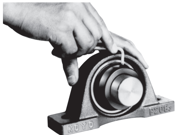
Fig. 14.10 Installing eccentric locking collar
