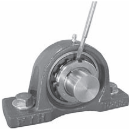
Fig. 14.8 Bending claw of washer (Locking locknut)
