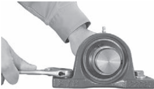
Fig. 14.4 Installation of setscrew units
