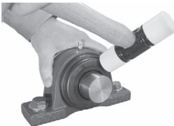
Fig. 14.13 Installing steel plate covers
