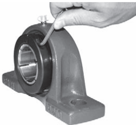
Fig 14.11 Installation of NU-LOC units
