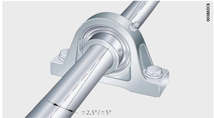
Figure 1 Compensation of static shaft misalignment
