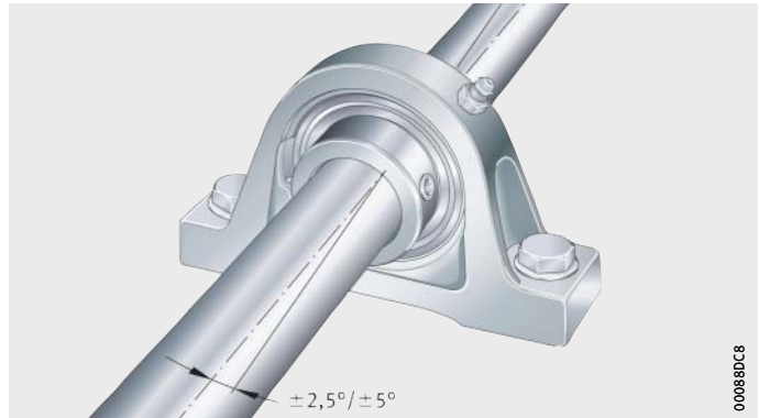
Figure 5 Compensation of static shaft misalignment
