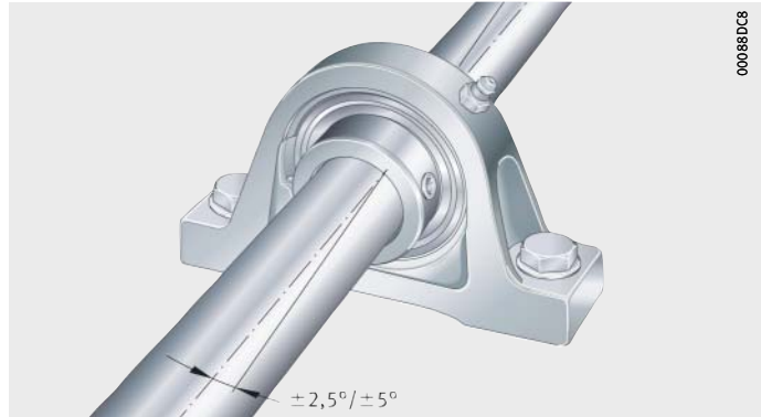
Figure 1 Compensation of static shaft misalignment
