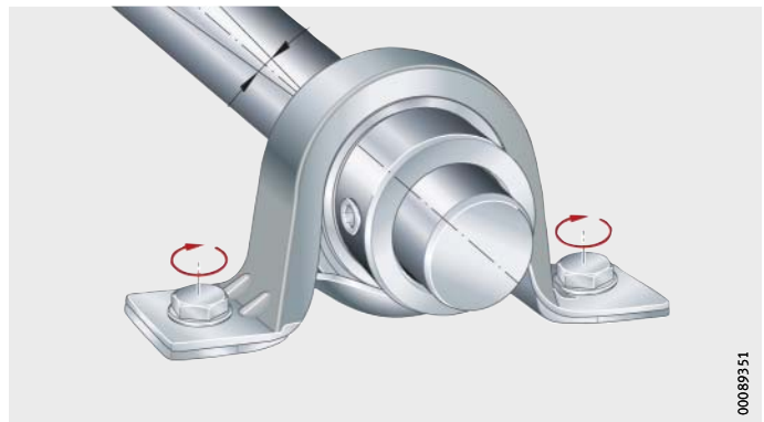
Figure 12 Screw mounting the housing finger tight
