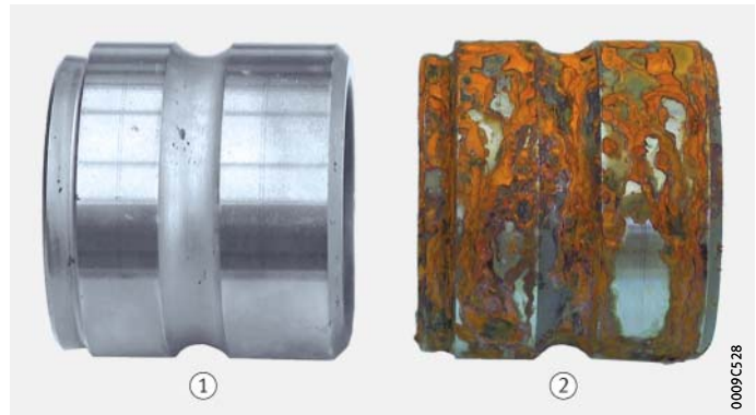
Figure 7 Coated and uncoated part after the salt spray test
