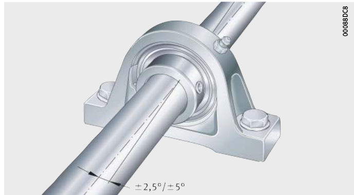
Figure 1 Compensation of static shaft misalignment
