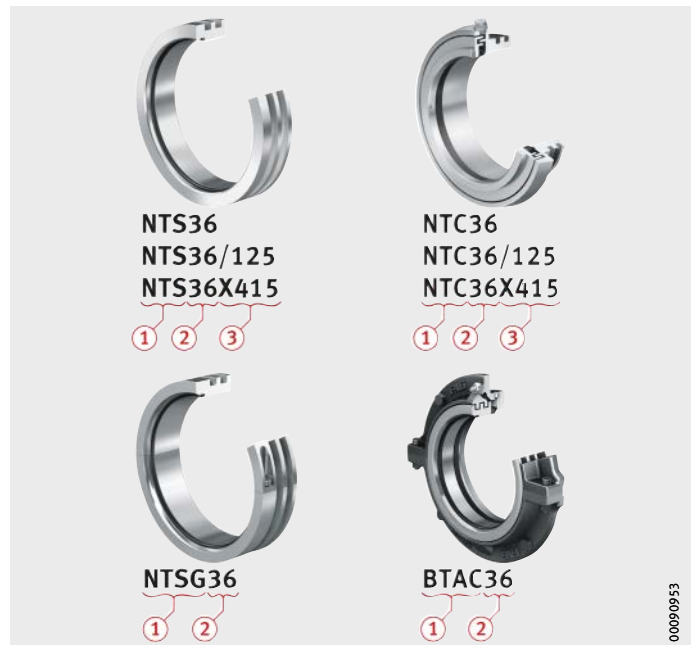
Figure 16 Designation structure of standard seals, examples
