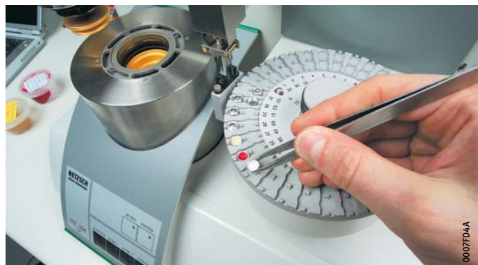
Figure 1 Analysis of the thermal behaviour of greases
