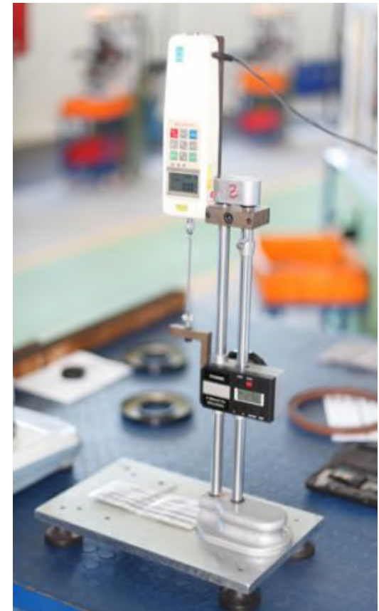
Spring Force Measurement
