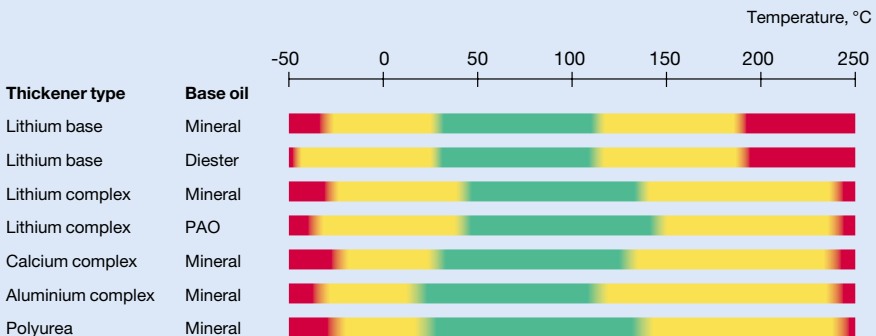
The SKF traffic light concept – standard greases
